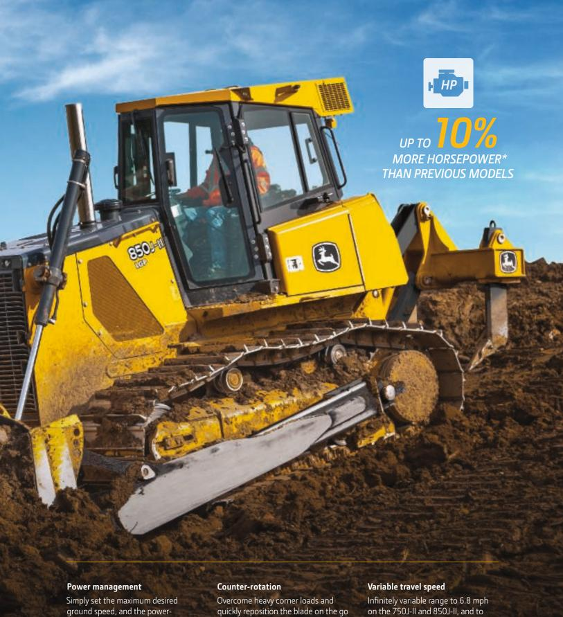
Simply set the maximum desired ground speed, and the power-management system automatically maintains peak engine rpm and power efficiency without stalling or shifting.
