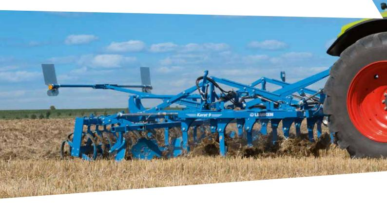
The Karat 9 intensive cultivator is available in working widths of 4 and 5 metres, of which the tines, are arranged on the cultivator frame with an average line distance of about 28 cm to achieve thorough mixing of soil and straw. The symmetrical tine arrangement effectively prevents lateral pull during work.
